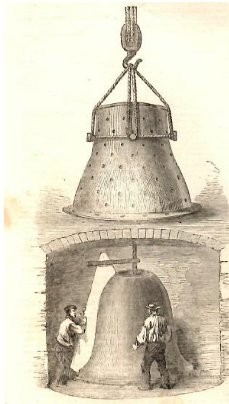
The Casting of the Bell, for the Great Clock of Westminster Palace, at Norton, Stockton-on-Tees from The Illustrated London News , 23 August 1856, page 194 (8.0cm by 15.0cm)
