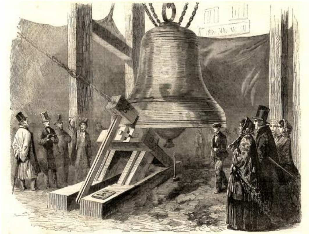
Experiment with the Hammer upon the Great Bell for the Westminster Clock from The Illustrated London News , 27 December 1856, page 639 (23.5cm by 18.5cm)
